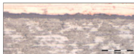
Zr-2.5%Nb sample tested 149 days: 2.5µm_x1000
