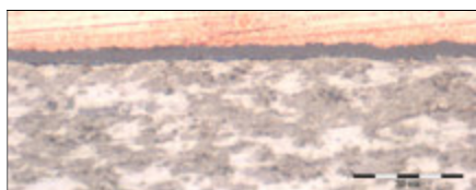
Zr-2.5%Nb sample tested 137 days: 2.4µm_x1000
