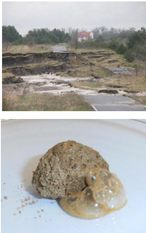
Fig. 17. Uncontrolled Formation of CO 2 in carbonate tests with original glacial till (left) [6] and Geotechnical incident in lignite opencast (right) [5].
