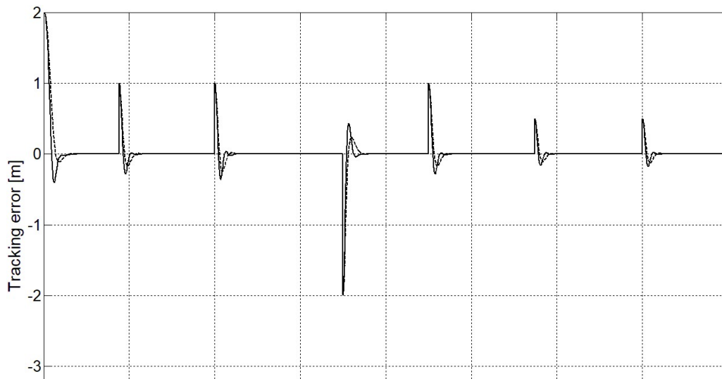
Fig. 5. Tracking error vs time in the proposed CS with staircase reference signal.
