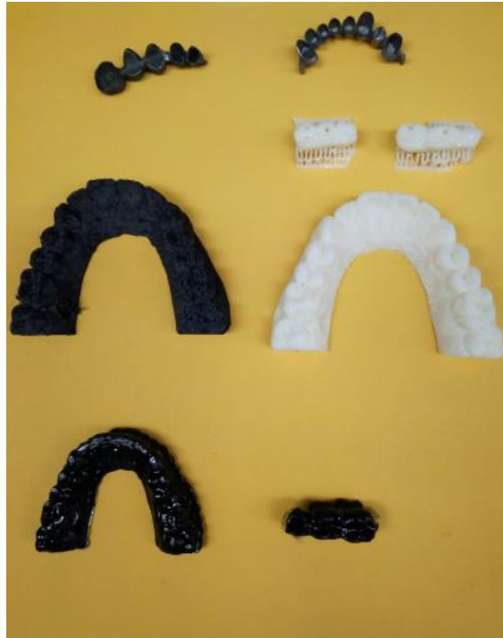
Fig.10 Realized dental prostheses and prosthetic dental models by three different technologies
