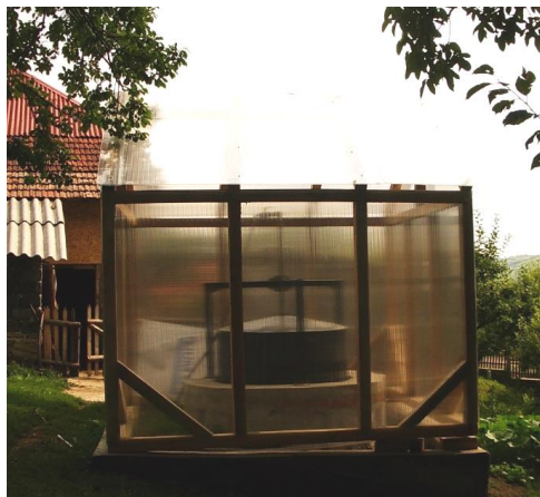
Fig. 4. Household biogas unit in operation in Boteni village, Argeş.
