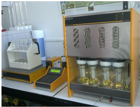
Fig. 2, a. Gerhardt Soxhlet fat extractor used for laboratory research.
