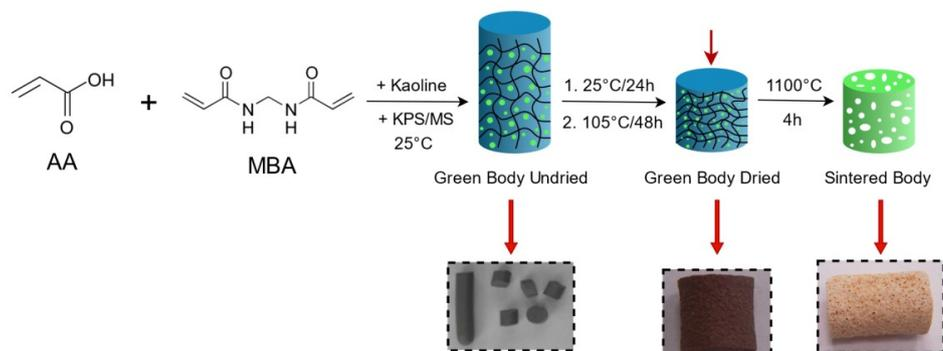
Fig. 1. Scheme for preparing ceramic foams.
