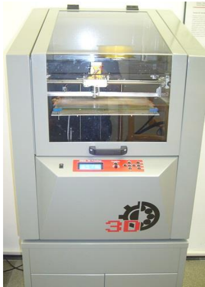
Fig. 1. 3D printer built at “Dunarea de Jos” University of Galati.
