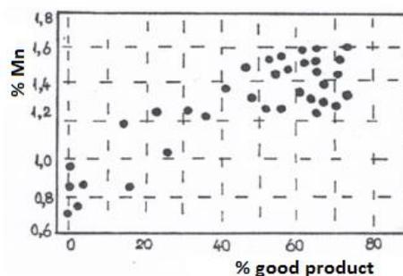
Fig. 2. Influence of the Mn content on the deformability of austenitic stainless steels.
