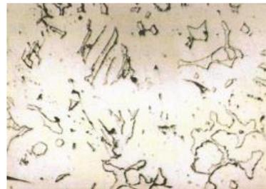
Fig. 16. Resulting microstructure after heating-up the samples according to diagram 7, Atac Nital 2%, 350 X
