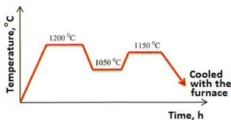
Fig. 3. Heating-up diagram 1
