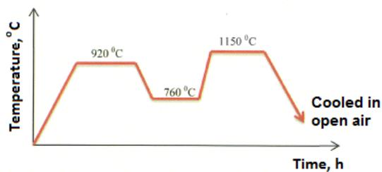
Fig. 5. Heating-up diagram 2
