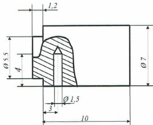
Fig. 19. Metallographic sample for the “Vacutherm” microscope
