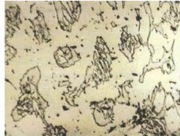
Fig. 14. Resulting microstructure after heating-up the samples according to diagram 6, Atac Nital 2%, 350 X
